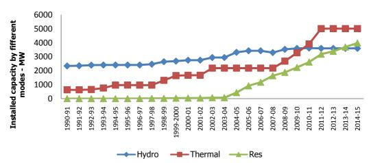
Figure 2: Installed Capacity (by modes) in Karnataka - MW
