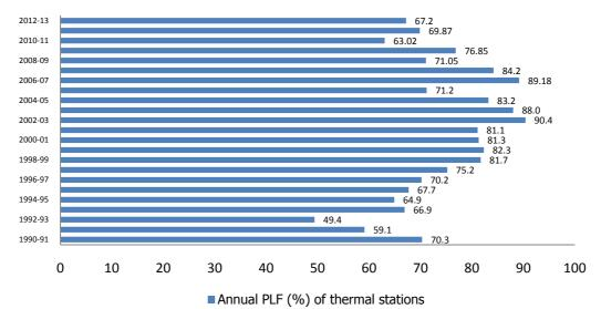
Figure 3: Annual Plant Load Factor (%) of Thermal stations in State sector in Karnataka
